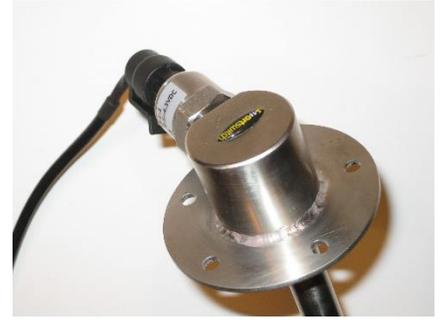
No drilling should be required to mount the sender assembly. The BEP sender has a  $\frac{3}{4}$  to 1-inch hole in the center which is sufficient to accept the “down tube” of the SEN sender assembly. Mounting holes should match.
